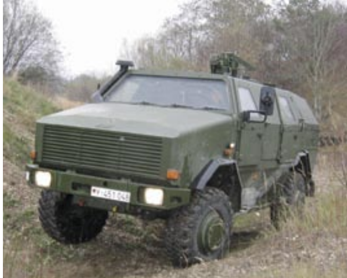
Krauss-Maffei Wegmann’s Dingo 2 all-protected vehicle has shielded crews against mines, IEDs and other threats.
